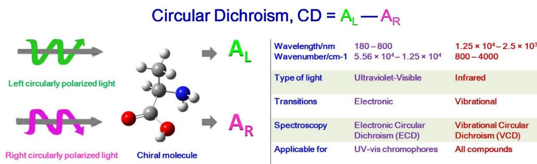
Fig. 2. Schematic description of CD,  $A_L$  and  $A_R$  are absorptions of left- and right-circularly polarized light.
