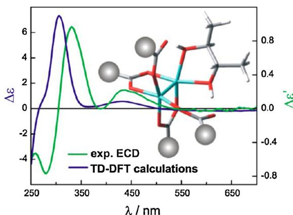
**Fig. 4.** Structure of dimolybdenum tetracarboxylate chelating vic-diol complex involved and their experimental and TD-DFT calculated ECD spectra. Reproduced with permission from Ref. [22]. Copyright 2013 American Chemical Society.
