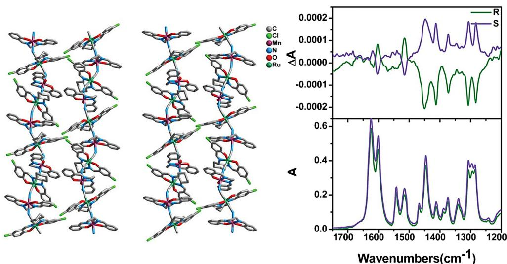
**Fig. 23.** Structures of 1-D zigzag Ru<sup>III</sup>-Mn<sup>III</sup> heterobimetallic chains derived from ((R,R) (left) and (S,S))- $[\text{Bu}_4\text{N}]^+[\text{Ru}(5\text{-Cl-Salcy})(\text{CN})_2]$  (right), and their measured solid state VCD and IR spectra in KBr pellets [115].
