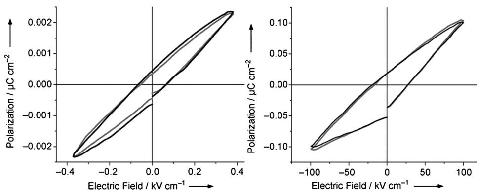
**Fig. 19.** Polarization hysteresis loops of europium complex **1** on powdered samples (left) and on thin films (right) [82].
