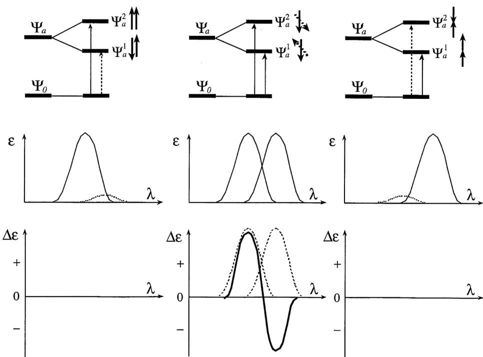
**Fig. 5.** Exciton coupling of two degenerate transitions, the absorption and ECD spectra: ground states ( $\Psi_0$ ), excited states ( $\Psi_a$ , split into  $\Psi_a^1$  and  $\Psi_a^2$  due to the interaction) [16(a)]. Reproduced with a permission of Elsevier.
