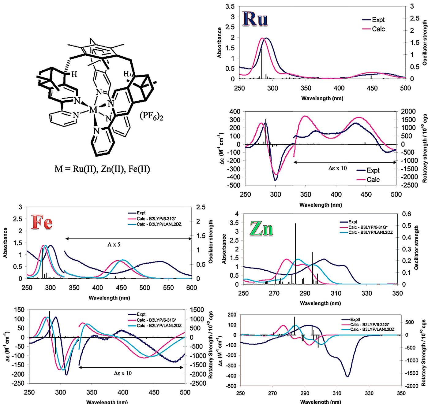
**Fig. 3.** The structures of chiral hemicage metal complexes and their corresponding experimental and calculated UV-vis and ECD spectra. Reproduced with permission from Ref. [21(c)]. Copyright 2008 American Chemical Society.
