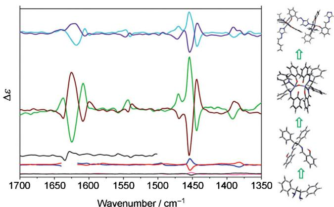
**Fig. 14.** VCD spectra monitoring the polymerization process, from bottom to top: chirality-pool diamine, Schiff base ligand, dinuclear iron(III) complex, and 1D iron(III) coordination polymer [69].
