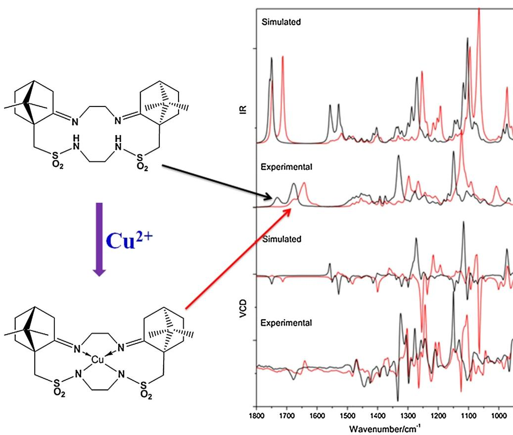
**Fig. 13.** Copper(II) coordination with a chiral ligand monitored by VCD [21(d)].
