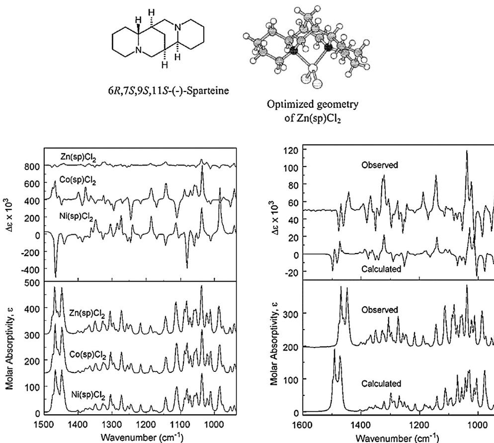
**Fig. 11.** Experimental VCD spectra of Zn(sp)Cl<sub>2</sub>, Co(sp)Cl<sub>2</sub>, and Ni(sp)Cl<sub>2</sub> (left) and simulated VCD spectra of Zn(sp)Cl<sub>2</sub> (right). Reproduced with permission from Ref. [42]. Copyright 2001 American Chemical Society.
