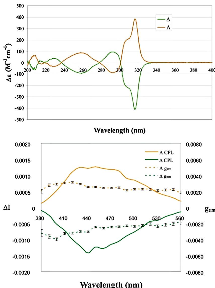
**Fig. 9.** The experimental ECD (up); and CPL spectra with the emission dissymmetry values (bottom) of Zn(II) hemicage complexes ( $\Delta$ -configuration, green; and  $\Lambda$ -configuration, orange). Reproduced with permission from Ref. [33]. Copyright 2007 American Chemical Society.
