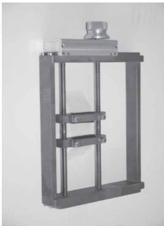
Figure 18.21. A mechanical film stretcher with oppositely threaded screws to ensure even stretching of the film. (See insert for color representation of the figure.)
