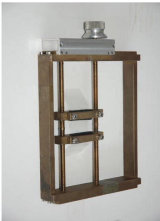
Figure 18.21. A mechanical film stretcher with oppositely threaded screws to ensure even stretching of the film. See page 515 for text discussion.
